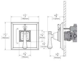
VALVE MOUNTING IS SHOWN FOR REFERENCE ONLY. VALVE IS NOT INCLUDED WITH CPT-8400-P
